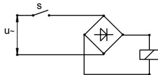
Fig. 51: Circuit diagram damping by mains rectifier
