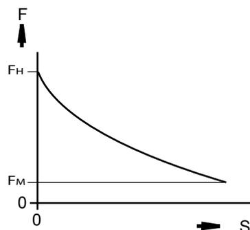
Fig. 49: Increasing characteristic
