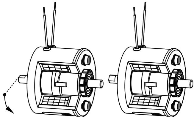
Fig. 10: Cross section ON/OFF rotary solenoid
