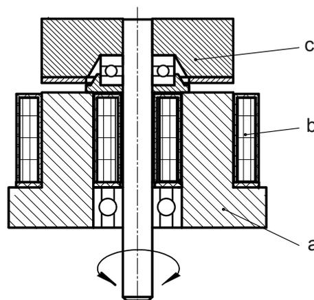
Fig. 13: Principle proportional rotary solenoid G DR
