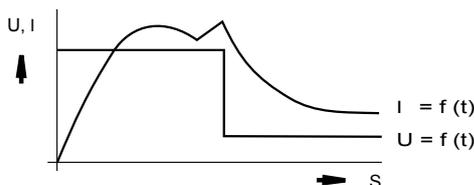
Fig. 34: Switch is actuated by delayed relay drive
