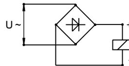
Fig. 45: Circuit diagram solenoid AC connection
