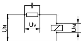
Fig. 35: Circuit diagram series resistor with capacitor
